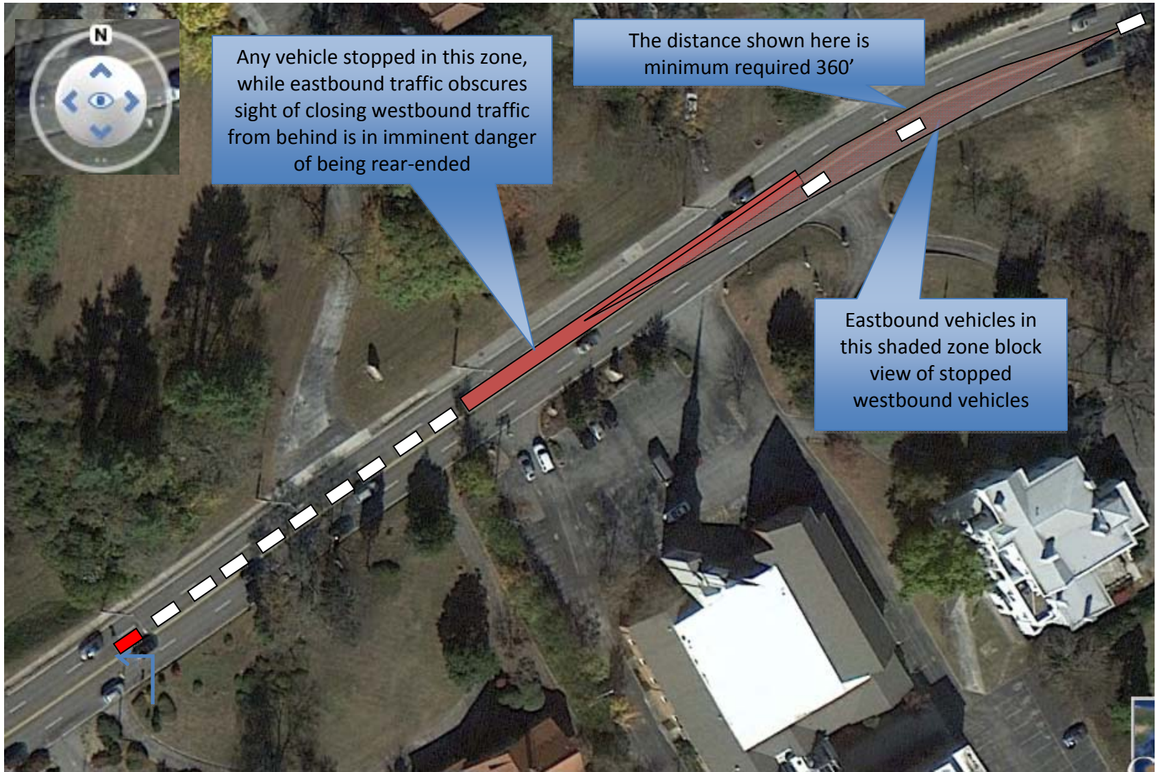
Figure 2. Stopping sight distance to safely stop behind queue of vehicles in inside lane
